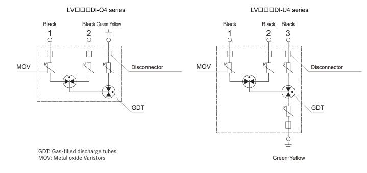
Flexible wires in black color can connect to each phase without any specific control.
